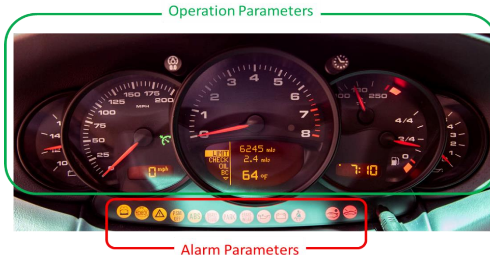
Figure 46: Instrument panel (dashboard) in a car, with operation parameters and alarm parameters.
