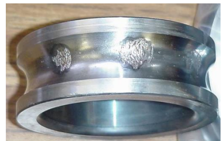
Figure 24: A damaged bearing, due to false brinelling.
