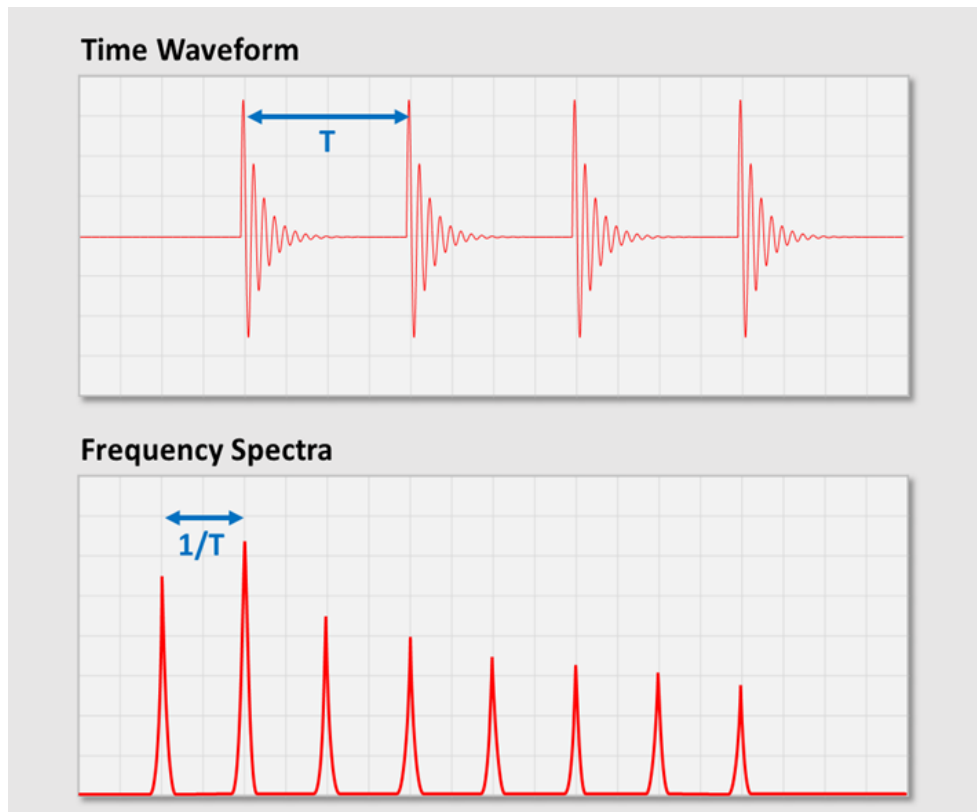
Figure 33: Illustration of the time period T in the Time Waveform, and the impact frequency 1/T in the Frequency Spectra.
