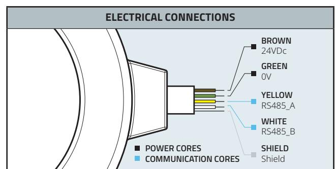
**NB.** The sensor shield must be connected to the system Common.
