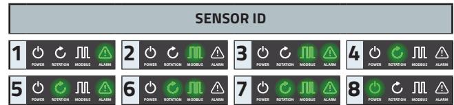
When the sensor is powered-up, the sensor LEDs will indicate the actual sensor ID no.
